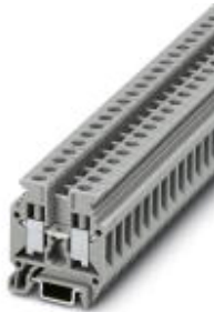
Feed-through terminal block, Connection method: Screw connection, Cross section: 0.2 mm 2 - 6 mm 2 , AWG 24 - 10, Width: 6.2 mm, Color: gray, Mounting type: NS 15
