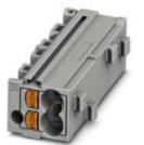
Marshalling patchboard, Nom. voltage: 500 V, Nominal current: 17.5 A, Cross section: 0.14 mm<sup>2</sup> - 2.5 mm<sup>2</sup>, AWG: 12 - 26, Connection type: Push-in connection, Number of positions: 1, Number of connections: 4, Width: 11 mm, Length: 8.6 mm, Color: gray, Color of connection elements: orange, Assembly: for snapping onto a DIN rail adapter, for snapping onto a cover flange
