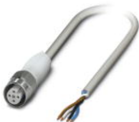
Sensor/Actuator cable, 4-position, PP-EPDM halogen-free, Gray RAL 7035. Free cable end, on Socket straight M12, A-coded, Cable length: 1.5 m, Hygienic design, With high-grade steel knurl
