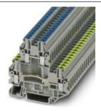
Feed-through terminal block, Connection method: Screw connection, Cross section: 0.14 mm² - 6 mm², AWG: 26 - 10, Width: 8.7 mm, Height: 64.4 mm, Color: gray, Mounting type: NS 35/7,5, NS 35/15
