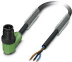
Sensor/Actuator cable, 3-position, PUR halogen-free, Black-gray RAL 7021, Plug angled M12, A-coded, on Free cable end, Cable length: 3 m, with plastic knurl
