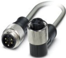
Bus system cable, DeviceNet, 5-position, PUR halogen-free, Gray RAL 7001, Plug straight 7/8"-16UNF, on Socket angled 7/8"-16UNF, Cable length: 5 m
