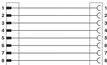
Contact assignment of the M12 connector and the M12 socket
