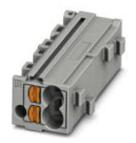
Marshalling patchboard, Nom. voltage: 500 V, Nominal current: 17.5 A, Cross section: 0.14 mm² - 2.5 mm², AWG: 12 - 26, Connection type: Push-in connection, Number of positions: 1, Number of connections: 4, Width: 11 mm, Length: 8.6 mm, Color: gray, Color of connection elements: violet, Assembly: for snapping onto a DIN rail adapter, for snapping onto a cover flange
