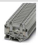
Disconnect terminal block, Connection method: Screw connection, Cross section: 0.5 mm<sup>2</sup> -10 mm<sup>2</sup>, AWG: 20 - 10, Width: 8.2 mm, Mounting type: NS 35/7,5, NS 35/15, NS 32, Color: gray
