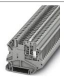
Knife disconnect terminal block, with actuation bracket and white disconnect knife, Connection type: Screw connection, Cross section: 0.14 mm² - 6 mm², AWG: 26 - 10, Nominal current: 20 A, Nominal voltage: 500 V, Length: 57.8 mm, Width: 6.2 mm, Color: gray, Assembly: NS 35/7,5, NS 35/15
