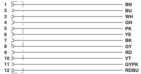
Contact assignment of the M12 socket
