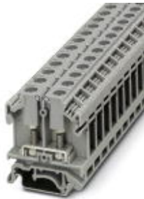
Universal terminal block with bolt connection, cross section: 0.1 - 6 mm 2 , width: 11 mm, color: Gray
