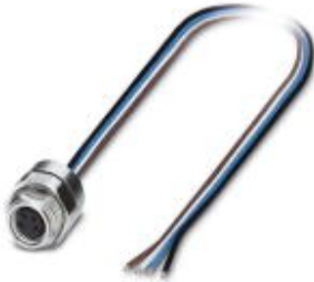
Sensor/actuator flush-type socket, 4-pos., M8, rear/screw mounting with M12 thread, with 0.5 m TPE litz wire, 4 x 0.25 mm 2
