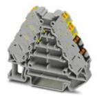
Potential distributors, Nom. voltage: 250 V, Nominal current: 17.5 A, Cross section: 0.14 mm² - 2.5 mm², AWG: 14 - 26, Connection type: Push-in connection, Width: 8.3 mm, Length: 64 mm, Color: gray, Assembly: NS 35/7,5, NS 35/15
