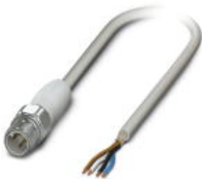
Sensor/Actuator cable, 4-position, PP-EPDM halogen-free, Gray RAL 7035, shielded, Plug straight M12, A-coded, on Free cable end, Cable length: 10 m, Hygienic design, With high-grade steel knurl
