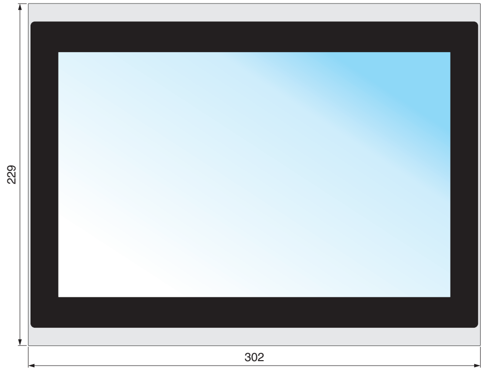
Figure 2-5 Front panel (dimensions in mm)
