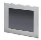
Touch panel with 30.7 cm/12.1" TFT-Display (Analog resistive (polyester)), 800 x 600 Pixel (SVGA), 262144 colors, ARM® Cortex®-A8, 800 MHz, 2x USB host 2.0, 1 x Ethernet (10/100 Mbps), RJ45, Windows® Embedded Compact 7 and User software: IniNet Browser. (Bus system: without)
