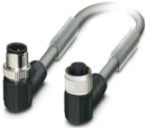
Bus system cable, CANopen®, 5-position, PUR halogen-free, Gray RAL 7001, shielded, Plug angled M12-SPEEDCON, A-coded, on Socket angled M12-SPEEDCON, A-coded, Cable length: 10 m
