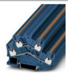
Double-level terminal block, Cross section: 0.14 mm<sup>2</sup> - 4 mm<sup>2</sup>, AWG: 26 - 12, Connection type: Push-in connection, Width: 5.2 mm, Color: blue, Mounting type: NS 35/7,5, NS 35/15
