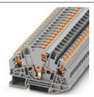
Test disconnect terminal block, nom. voltage: 1000 V, nominal current: 30 A, connection method: Push-in connection, Rated cross section: 6 mm², cross section: 0.5 mm² - 6 mm², color: gray
