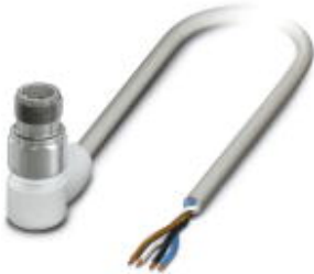
Sensor/Actuator cable, 4-position, PP-EPDM halogen-free, Gray RAL 7035, Plug angled M12, A-coded, on Free cable end, Cable length: 10 m, Hygienic design, With high-grade steel knurl
