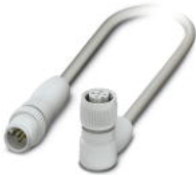
Sensor/Actuator cable, 5-position, PP-EPDM halogen-free, Gray RAL 7035, Plug straight M12, A-coded, on Socket angled M12, A-coded, Cable length: 0.6 m, Hygienic design, with plastic knurl
