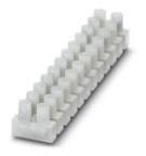
Polyamide Europe terminal strip, transparent, for connecting solid conductors and stranded conductors with ferrules with a cross section of 1 to 10 mm<sup>2</sup>
