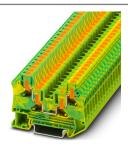
Ground modular terminal block, number of connections: 2, number of positions: 1, connection method: Push-in connection, Rated cross section: 6 mm², cross section: 0.5 mm² - 10 mm², mounting type: NS 35/7,5, NS 35/15, color: green/yellow
