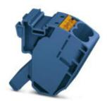
Pick-off terminal block, Connection method: Push-in connection, Cross section: 0.5 mm² - 16 mm², AWG: 20 - 6, Width: 18.5 mm, Height: 34.7 mm, Color: blue, Mounting type: On base element
