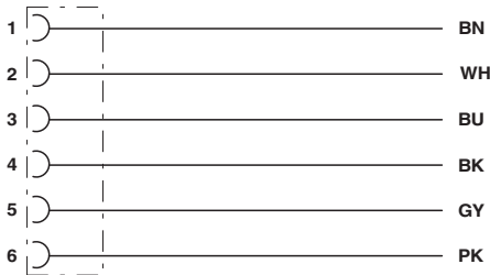
Contact assignment of M8 socket
