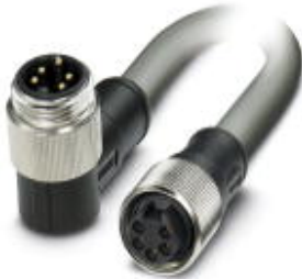
Bus system cable, DeviceNet, 5-position, PVC, Gray RAL 7001, Plug angled 7/8"-16UNF, on Socket straight 7/8"-16UNF, Cable length: 2 m
