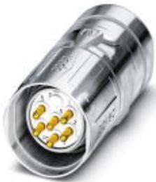
Cable connector, straight, shielded: yes, SPEEDCON locking, M23, Number of positions: 6, Type of contact: Male connector, Crimp connection, Cable diameter: 10 mm ... 14.5 mm
