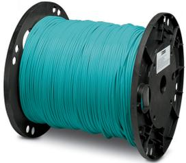
By the meter, Cable reel, Ethernet CAT5 (100 Mbps), shielded, TPE, Teal, 8-wire (4x2xAWG24/7; SF/UTP), color single wire: white/blue-blue, white/orange-orange, white/green-green, white/brown-brown, cable length: 300 m, highly flexible
