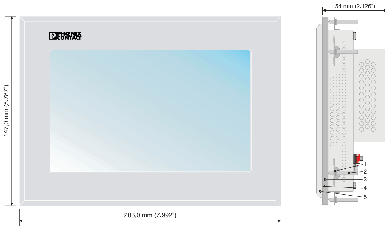
Figure 4 Front view of the TP 07T with dimensions
