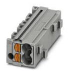
Marshalling patchboard, Nom. voltage: 500 V, Nominal current: 17.5 A, Cross section: 0.14 mm² - 2.5 mm², AWG: 12 - 26, Connection type: Push-in connection, Number of positions: 1, Number of connections: 4, Width: 11 mm, Length: 8.6 mm, Color: gray, Color of connection elements: pink, Assembly: for snapping onto a DIN rail adapter, for snapping onto a cover flange
