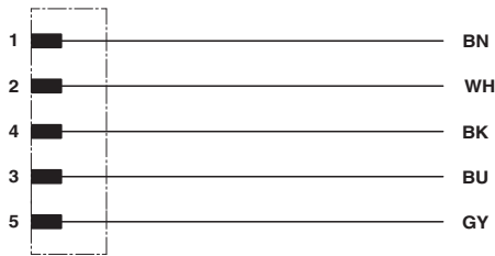
Contact assignment of the M12 plug
