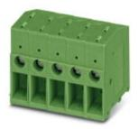
PCB terminal block, Nominal current: 32 A, Nom. voltage: 630 V, Pitch: 7.62 mm, Number of positions: 3, Connection method: Screw connection, Mounting: Soldering, Conductor/PCB connection direction: 0 °, Color: green, The article can be aligned to create different nos. of positions!
