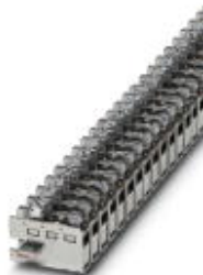
Power terminal block, Connection method Screw connection, Load current : 125 A, Cross section: 0.75 mm 2 - 35 mm 2 , Width: 12 mm, Color: aluminum
