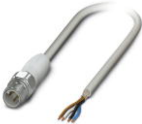
Sensor/Actuator cable, 4-position, PP-EPDM halogen-free, Gray RAL 7035, shielded, Plug straight M12, A-coded, on Free cable end, Cable length: 5 m, Hygienic design, With high-grade steel knurl
