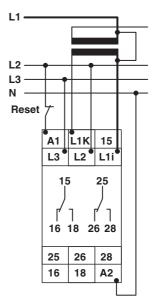
$3 \sim 400 \text{ V}$  measuring range, with error memory, 230 V AC supply voltage,  $I_N > 10 \text{ A}$
