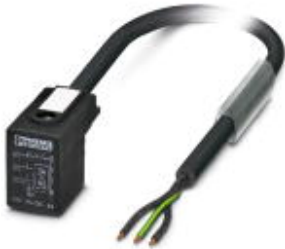
Sensor/Actuator cable, 3-position, PUR halogen-free, Black-gray RAL 7021, Free cable end, on BI valve plug (11 mm), with 1 LED, connected with Z diode, Cable length: 10 m
