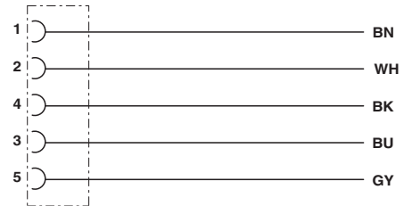
Contact assignment of the M12 socket
