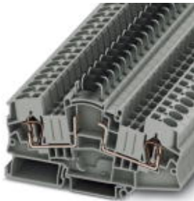
Component terminal block, Connection method: Spring-cage connection, Cross section: 0.2 mm 2 -10 mm 2 , AWG: 24 - 10, Width: 8.2 mm, Color: gray
