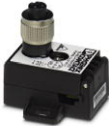
AS-Interface distributor with IP65/IP67/IP69k degree of protection for 1 flat-ribbon conductor, with a straight, A-coded, 2-pos. M12 socket
