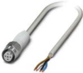
Sensor/Actuator cable, 4-position, PP-EPDM halogen-free, Gray RAL 7035, shielded, Free cable end, on Socket straight M12, A-coded, Cable length: 3 m, Hygienic design, With high-grade steel knurl
