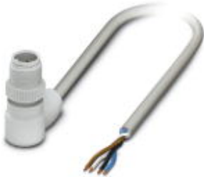
Sensor/Actuator cable, 4-position, PP-EPDM halogen-free, Gray RAL 7035, Plug angled M12, A-coded, on Free cable end, Cable length: 3 m, Hygienic design, with plastic knurl
