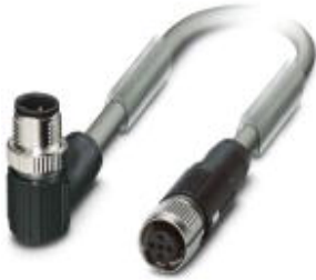
Bus system cable, CANopen®, 5-position, PUR halogen-free, Gray RAL 7001, shielded, Plug angled M12-SPEEDCON, A-coded, on Socket straight M12-SPEEDCON, A-coded, Cable length: 0.3 m
