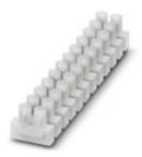
Polyamide Europe terminal strip, transparent, for connecting solid conductors and stranded conductors with ferrules with a cross section of 0.75 to 6 mm<sup>2</sup>
