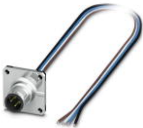
Sensor/Actuator flush-type plug, 4-pos., M12, A-coded, front/square flange mounting, with 0.5 m TPE litz wire, 4 x 0.34 mm 2
