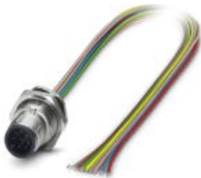
Sensor/actuator flush-type connector, 8-pos., M12-SPEEDCON, rear/screw mounting with Pg9 thread, with 0.5 m TPE litz wire, 8 x 0.25 mm 2
