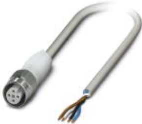
Sensor/Actuator cable, 4-position, PP-EPDM halogen-free, Gray RAL 7035, Free cable end, on Socket straight M12, A-coded, Cable length: 5 m, Hygienic design, With high-grade steel knurl
