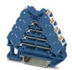
Marshalling panel, Nom. voltage: 250 V, Nominal current: 10 A, Cross section: 0.14 mm² - 2.5 mm², AWG: 12 - 26, Connection type: Push-in connection, Width: 8.3 mm, Length: 64 mm, Color: blue, Assembly: NS 35/7,5, NS 35/15
