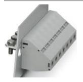
Panel feed-through terminal block, Connection method: Screw connection, Bolt connection, Load current : 150 A, Cross section: 16 mm<sup>2</sup> - 50 mm<sup>2</sup>, AWG 6 - 1/0, Connection direction of the conductor to plug-in direction: 90 °, Width: 18.8 mm, Color: gray
