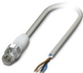
Sensor/Actuator cable, 4-position, PP-EPDM halogen-free, Gray RAL 7035, Plug straight M12, A-coded, on Free cable end, Cable length: 3 m, Hygienic design, With high-grade steel knurl
